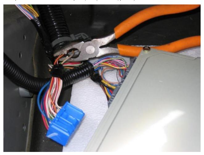
In this photo I show the speedo cable. Although the wiring may look as if it's being cut next to the ECU, in fact the wire is being cut between the point at which it enters the passenger footwell from the engine bay in a big bundle of cables (in the background) and the blue connector in the photo.
